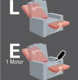
seperate adjustment of the backrest and leg rest by shifting the body
